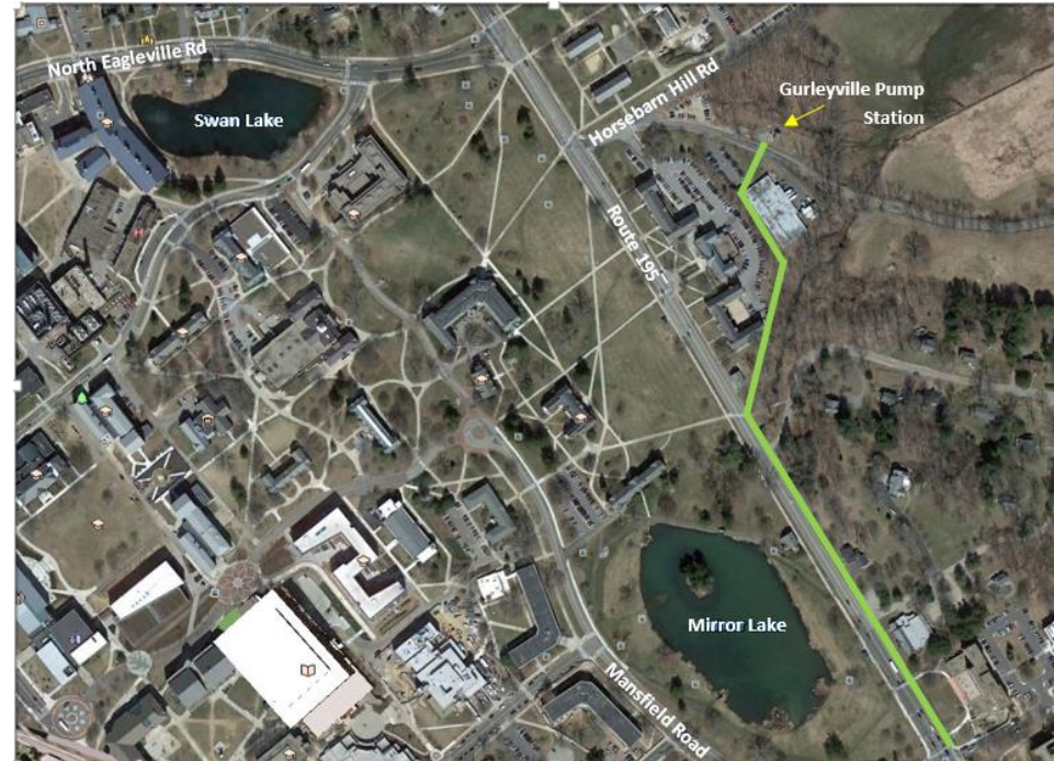
Sewer pipe location along 195 and behind residence halls
